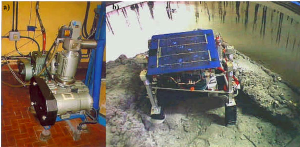
Fig. 6: Test bench used to perform tests in vacuum; a) vacuum pump, b) Walkie 6.2 in the vacuum camera.
